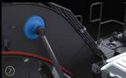
⑦ Reinforced boom cylinder cast bearing
